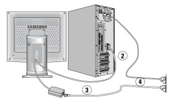
Figure 3. Cable connections (Analog)
